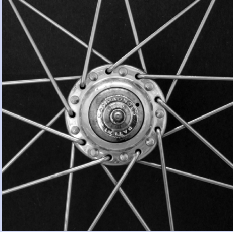
Narrow bike hub flanges (left) provide enough torsional rigidity for riders, while wide flanges (right) require more material, thus they add weight and cost.
